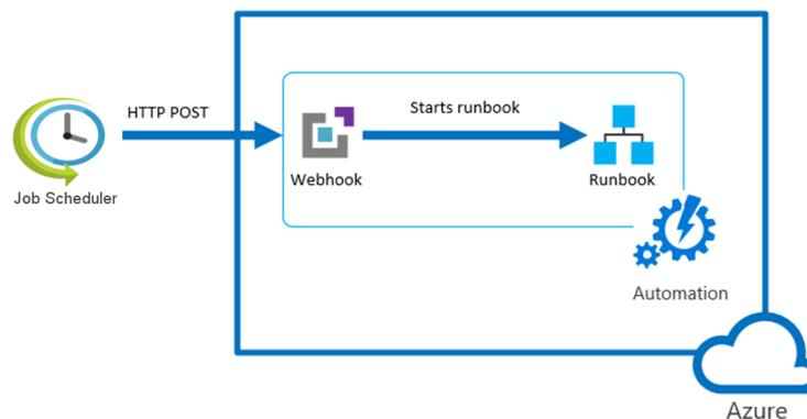
Figure 6-4 Concept of automated task [18][19]
