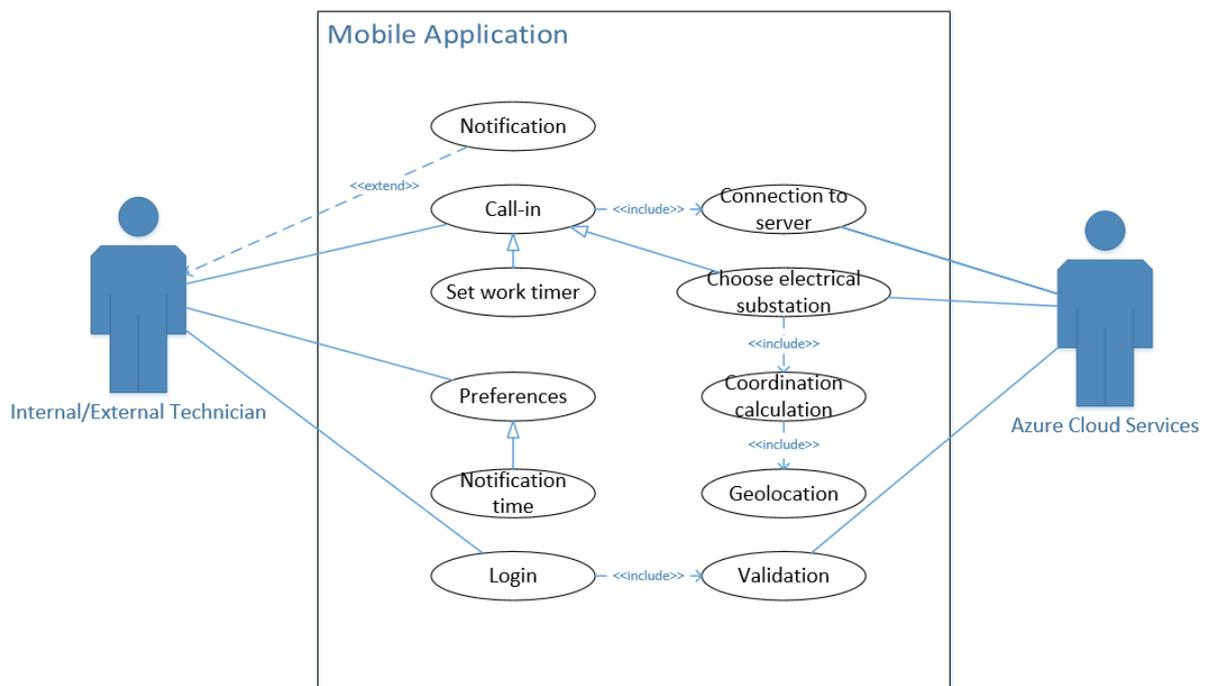
Figure 4-1 Use case diagram for mobile
